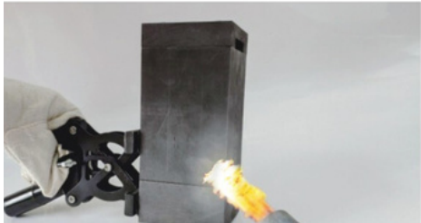
Preheat mold and conductor
