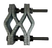
Supplied with 2 stainless steel threaded rods A2 10x100, A2 M10 stainless steel plate washers Side tightening in X fixing brackets are used to fix FRANKLIN France Early Streamer Emission and simple lightning conductors equipped with elevation rods or no on towers, vertical pipes, metal frameworks, etc....
